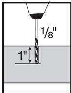
Drill down the depth shown into board at correct locations using bit size shown.
