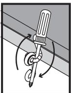
Screw hardware into board or ground using shaft of screwdriver for better leverage.
