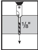
Drill through board at correct location with countersink tool and bit size shown.
