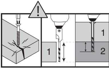
CAUTION: These boards should be pre-drilled and countersunk to avoid cracking. **Note: Adjust countersink tool to width of first board to countersink to proper depth. Pre-drill into second board using first board as a template before attaching.**
