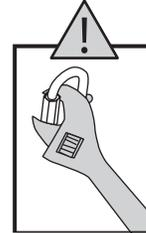
CAUTION: Use wrench to tighten Quick-Link Connectors. Failure to tighten Quick-Links securely could result in injury.
