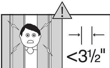
CAUTION: Spacing between boards must be less than 3 1/2" (or greater than 9") or a head/neck entrapment could exist.
