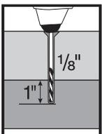
Pre-drill into second board with correct depth and bit size shown.
